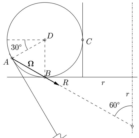
$$\left. \begin{aligned} \mathbf{v}_C^{\text{esfera}} &= \Omega \left( \frac{\sqrt{3}}{2} \mathbf{i} - \frac{1}{2} \mathbf{j} \right) \wedge (R \mathbf{i} + R \mathbf{j}) = \Omega R \left( \frac{\sqrt{3}}{2} + \frac{1}{2} \right) \mathbf{k} \\ \mathbf{v}_C^{\text{cilindro}} &= \omega r \mathbf{k} \end{aligned} \right\} \Rightarrow \boxed{\Omega = \omega}$$
